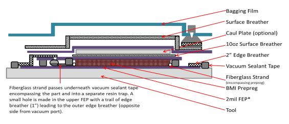
\*FEP is optional if the tool/mold is coated with a release agent
