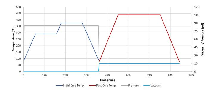
Note: This resin system requires a high-temperature post-cure to obtain optimal mechanical performance. Alternate postcure temperatures and hold times may be used to tune the system's Tg and toughness properties; please contact Toray CMA for more information.
